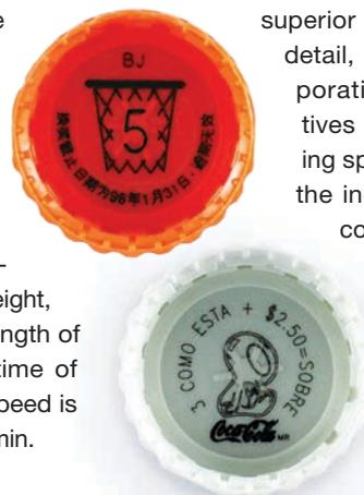
**FIGURE 4. On-the-fly laser marking of high-density polyethylene (HDPE) undercap promotions on linerless beverage closures enables up to 2000 closures/min.**
