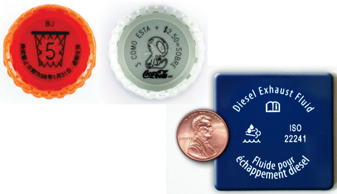
Photo B. Thermal chemical carbonization laser marking – “dark-colored” contrast on HDPE undercap promotions linerless beverage closures (left), and “light-colored” contrast on nylon automotive exterior/underhood components (right).
