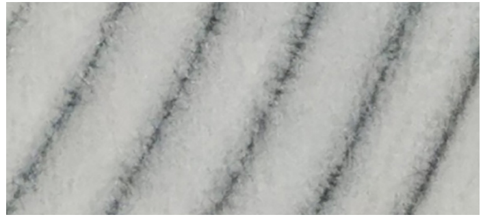
Figure 8. Textured ridges in the ABS plaque enhanced adhesion
