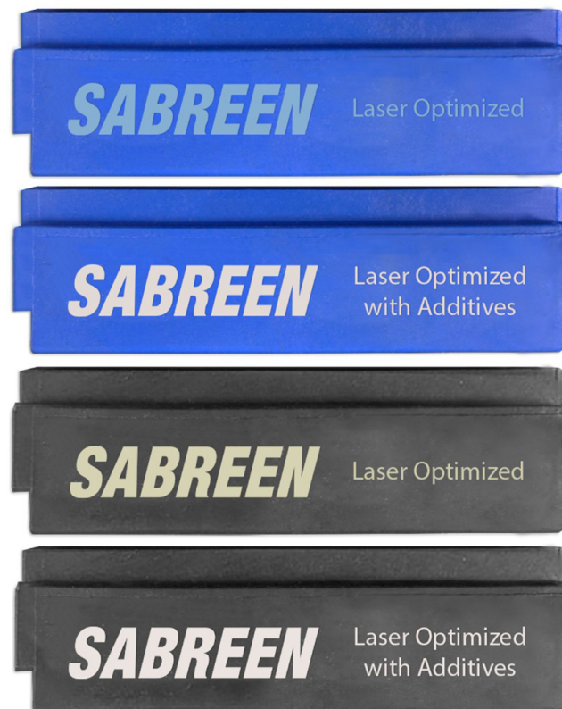
Image 1. Nylon laser marking color contrast on 20% glass-fill, matte surface texture
