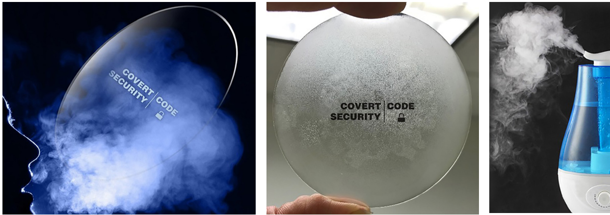
Figure 2. Permanent, invisible micro-etched codes temporarily appear when vapor is applied by mist, then rapidly disappear as moisture evaporates (left and middle). At the right is a vapor mist example. Photos courtesy of The Sabreen Group.
