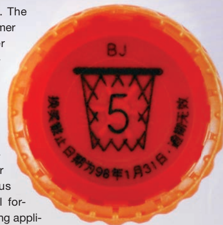
FIGURE 3. Laser marking undercap promotions on linerless beverage closures at speeds up to 1,500 per minute.
